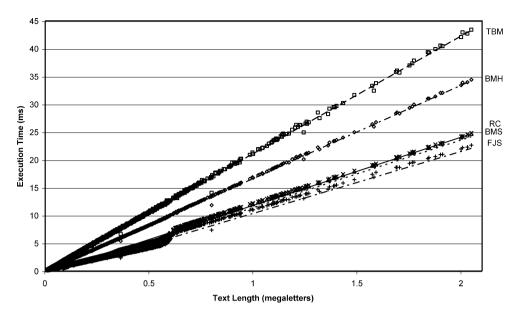
Fig. 2. Execution time versus text length for moderate-frequency pattern set.
