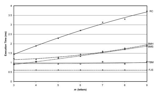
Fig. 6. Execution time versus pattern length for  $\mathbf{x} = a^{100\,000}$ ,  $\mathbf{p} = a^{m}$ .
