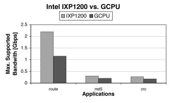
Fig. 11. Maximum supported bandwidth for Intel IXP1200 and a general-purpose processor similar to Intel Pentium III.
