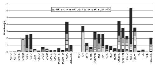
Fig. 7. Level-1 instruction cache miss ratios for different sizes of the cache.
