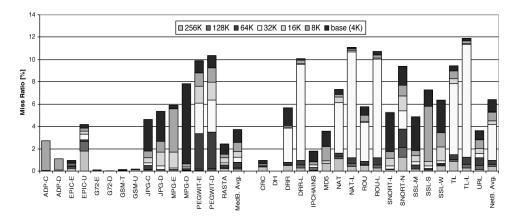
Fig. 6. Level-1 data cache miss ratios for different sizes of the cache.
