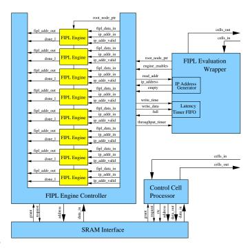
Fig. 12. Block diagram of FIPL evaluation environment.
