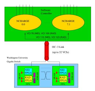
Fig. 9. Detail of the hardware and software components that comprise the FPX system. Each FPX is controlled by an NCHARGE software process. The contents of the memories on the FPX modules can be modified by remote processes via the software API to NCHARGE.
