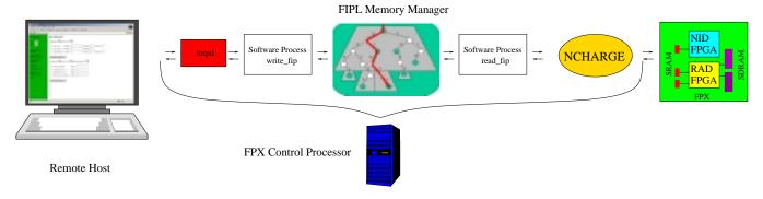
Fig. 10. Data flow with FIPL and NCHARGE
