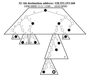
Fig. 3. IP lookup table represented as a multibit trie. A stride, 4-bits, of the unicast destination address of the IP packet are compared at once, speeding up the lookup process.
