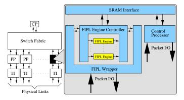
Fig. 6. Block diagram of router with multi-engine FIPL configuration; detail of FIPL system components in the Port Processor (PP).
