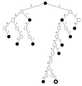
Fig. 2. IP lookup table represented as a binary trie. Stored prefixes are denoted by shaded nodes. Next hops are found by traversing the trie.
