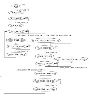
Fig. 8. FIPL engine finite-state-machine bubble diagram.
