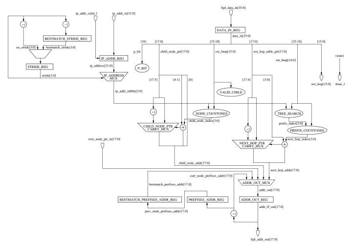
Fig. 7. FIPL engine dataflow; multi-cycle path from DATA IN FLOPS to ADDR OUT FLOPS can be scaled according to target device speed; all multiplexor select lines and flip-flop enables implicitly driven by finite-state machine outputs.
