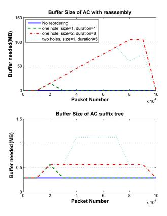
Figure 11: Buffer size while processing packets with Long Set
