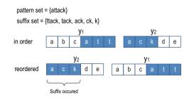
Figure 6: Examples of two packets' reordering
