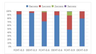
Fig.8.Off-chip memory accesses of DEHT and FCHT under various load factors with random inputs.
