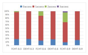
Fig.9. Off-chip memory accesses of DEHT and FCHT under various load factors with inputs of 80% true elements.
