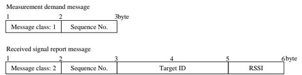
Figure 3. Packet formats of localization system.
