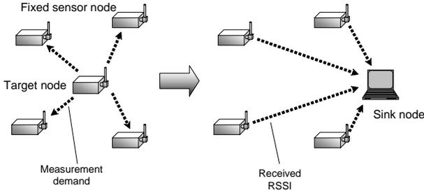
Figure 1. Localization system using RSSI measurement in sensor network.
