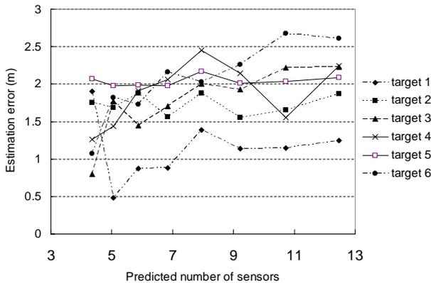
Figure 7. Relationship between predicted number of collectable data and position estimation error.
