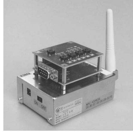
Figure 2. Ubiquitous Device equipped with the optional serial port.
