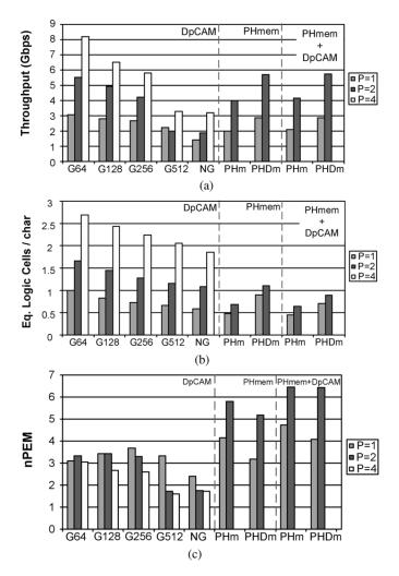
Fig. 11. PHmem and DpCAM performance, area cost, and efficiency. Memory area is calculated based on the following equation:  $12 \times MEMbytes =$  Logic Cell. (a) DpCAM and PHmem performance. (b) DpCAM and PHmem area cost. (c) DpCAM and PHmem efficiency.
