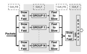
Fig. 5. DpCAM with multiple clock domains. Long, wide but slower busses (depicted with thick lines) distribute input data over large distances to the multiple search matching groups. These groups operate at higher clock rates to produce results faster.
