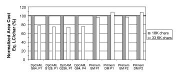
Fig. 12. Normalized area cost per matching character of different PHmem, DpCAM designs that match 18 and 33.6 K pattern characters. The values are normalized to the designs that match 18 K characters.
