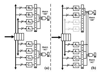
Fig. 1. Basic discrete comparator structure and its optimized version which shares common character comparators.
