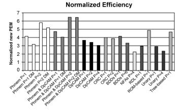
Fig. 13. Normalized nPEM of PHmem, DpCAM and related work. The performace of designs implemented in devices other than Virtex2 are normalized as follows. Spartan3:  $\times$  1.2; Virtex2Pro:  $\div$  1.25[8], [19], [24], [27].
