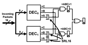
Fig. 4. DpCAM processing two characters per cycle.
