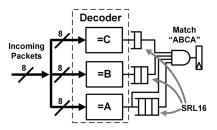
Fig. 2. Decoded CAM: Three comparators provide the equality signals for characters A, B, and C ("A" is shared). To match pattern "ABCA" we have to remember (using shift registers) the matching of character A, B, C, for 3, 2, and 1 cycles, respectively, until the final character is matched.
