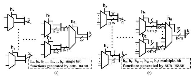
Fig. 7. Perfect hash trees: the select of each multiplexer is a function generated by the SUB\_HASH. (a) Binary hash tree. (b) Optimized hash tree.
