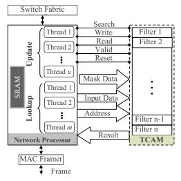
Figure 1(b) The proposed TCAM coprocessor/network processor.
