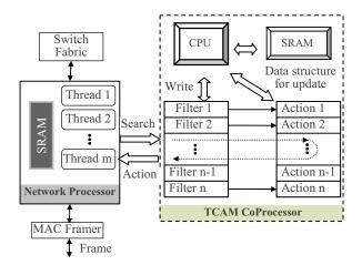
Figure 1(a) A conventional TCAM coprocessor/network processor.
